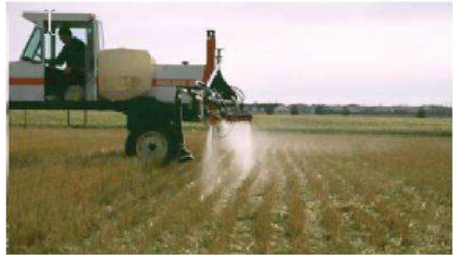
Figure 3. Air induction nozzles at 70 psi. (Wolf)
